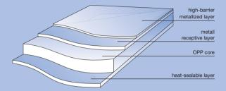
Treofan MPB is a biaxially oriented, co-extruded polypropylene film. Treofan MPB gives enhanced light and very high moisture and oxygen barrier. With its excellent metal adhesion it allows extrusion as well as adhesive lamination. Its heat-sealable layer on the non-metallized face provides good heat-seal integrity. Reels are normally wound with the metallized face on the outside, but can sometimes be supplied on request with the metallized face wound inside.
