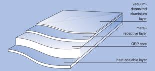
Treofan MNM is a biaxially oriented, co-extruded polypropylene film. Treofan MNM gives excellent light, moisture and odour barrier. With its excellent metal adhesion it allows high laminate bond strengths. Its heat-sealable layer on the non-metallized face provides good heat-seal integrity. The unmetallized version Treofan MND is sometimes available. Reels are normally wound with the metallized face on the outside, but can sometimes be supplied on request with the metallized face wound inside.
