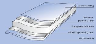
Treofan CLH has been especially designed for the holograms market and for lamination with paper, carton and plastic films. Treofan CLH is also a suitable support for vacuum metallization.
