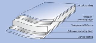
Treofan CLG has been especially designed to merge the aesthetic and protection properties of the acrylic-coated film with outstanding machinability performances.
